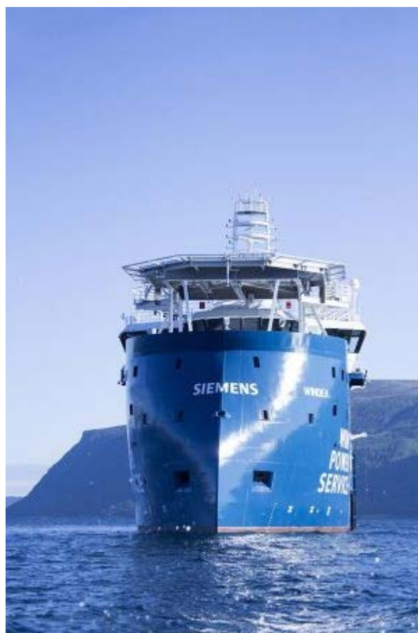
Ulstein X-Bow is based on an inverter bow concept
